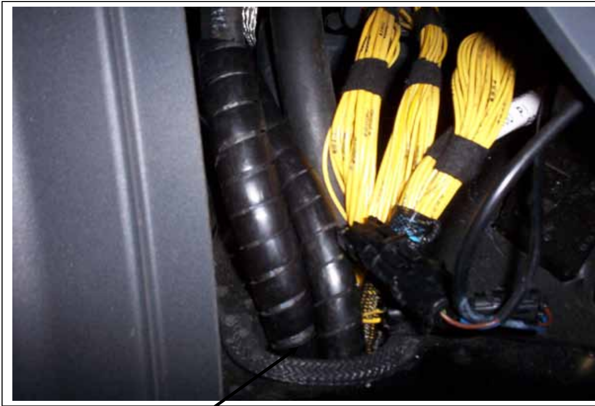
1/2" hose to evaporator coil
