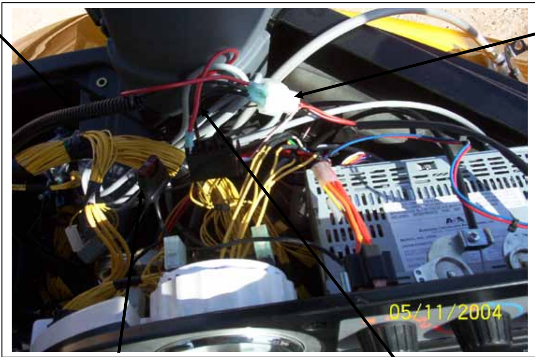
Inline ATO fuse holder between blower switch and A/C on-off push button
