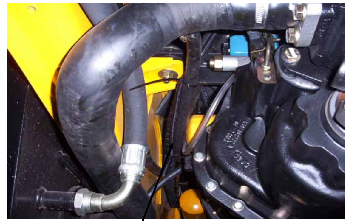
1/2" line and clutch wire coming from compressor down and back towards the right hand side of the cab.
