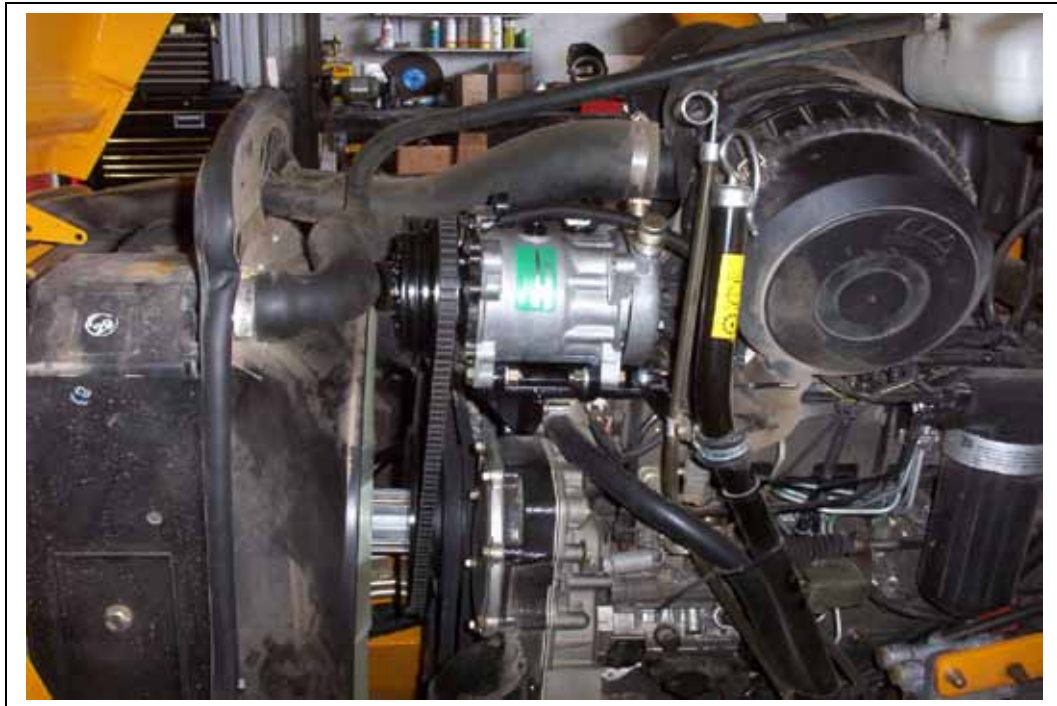
Compressor installed on mount
