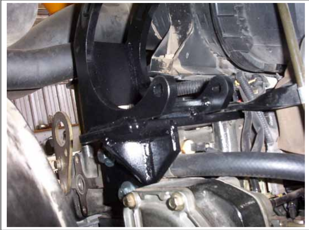
Side view mount bolted in place
