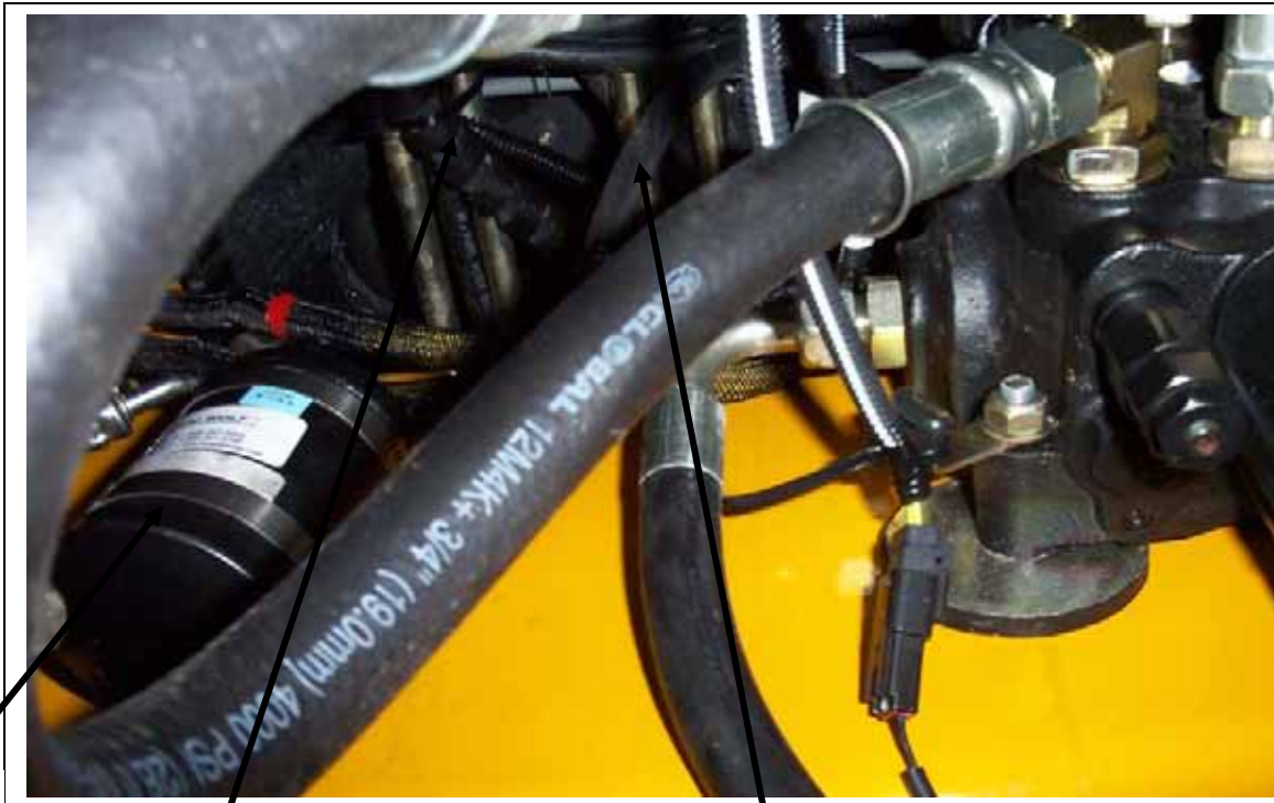
1/2" line and clutch wire coming from compressor down and back towards the right hand side of the cab.
